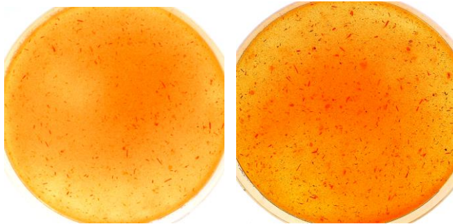
MF=Medium Finish (0.033-0.045”) CF=Coarse Finish (0.045-0.060”)
